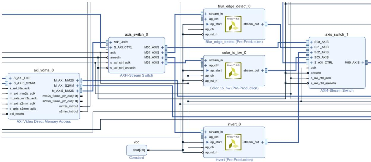
Figure 5: Video Stream Mux/Demux
