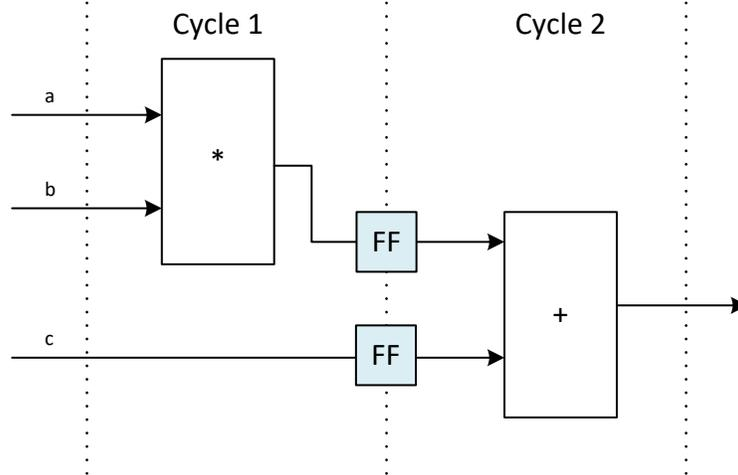
Figure 2: Pipelined Execution
