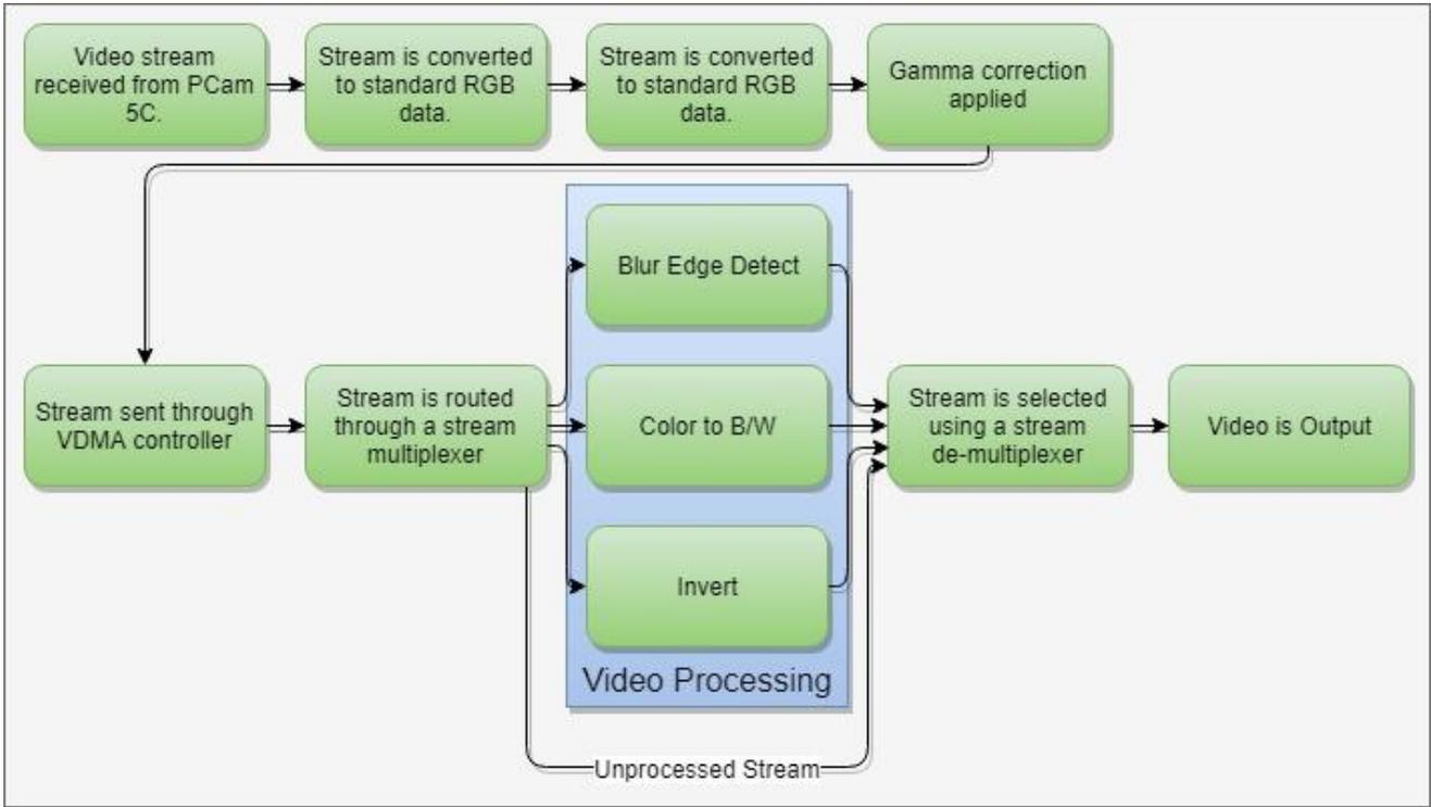
Figure 3: Video Pipeline Operation Flowchart
